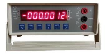
With good long-term stability and small temperature coefficient, this voltagecurrent meter is very suitable for voltage measurement of DC resistors and calibration of voltage and current sensors. The voltage measuring accuracy is  $\pm 0.01\%$  and the current measuring accuracy is  $\pm 0.05\%$ .
