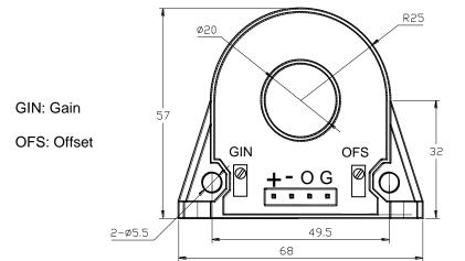
Terminal +: +15V, Terminal -: -15V, Terminal O: Output, Terminal G: ground
