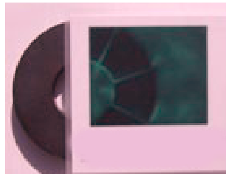
Detecting the multi-poles of a ring magnet
